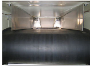
Full length adjustable skirt boards
